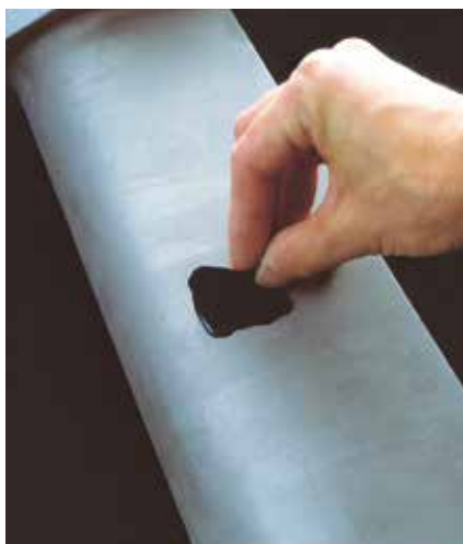
An operator peels off the cured replica
