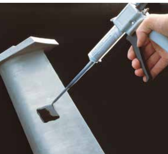
An operator dispenses RepliSet onto a sample
