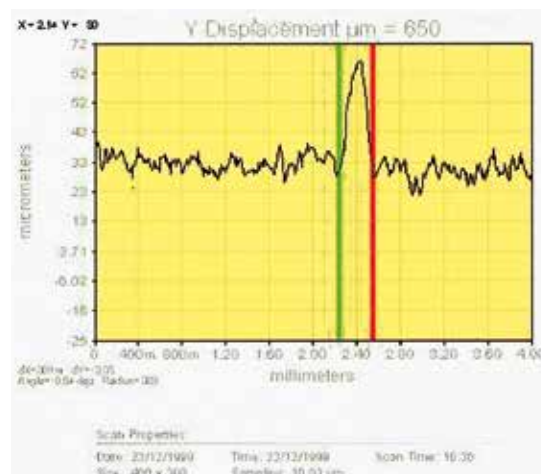
Depth of pitting
